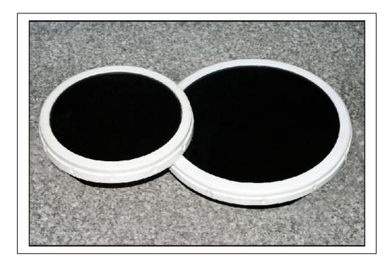
Fine Bubble PROFLEX membrane DISC diffusers are compression moulded and made with less than 10% extractable oils to ensure exceptional quality, strength and longer product life. The base and retaining ring are designed to seal tightly and made of polypropylene having properties of higher temperature resistance and greater ductility.
